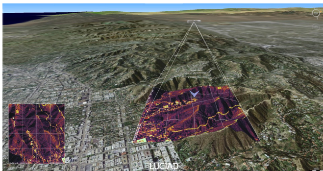
Figure 3 - Real-time video draping from UAV feed
