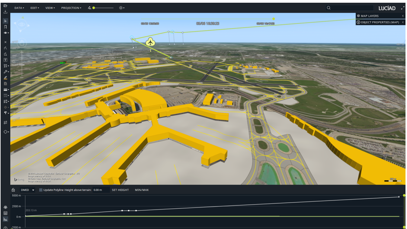
Figure 11 - AIXM5 data and flight plan preview in 3D with vertical view.
