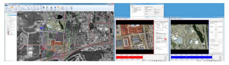
Graphic displays of full motion video and its associated tracking graphics are geofused with other forms of geospatial information to provide an instant view of the common operating picture
