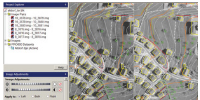
MicroStation design file graphics are displayed by PRO600 in full 3D stereo.
