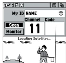
*The Code field will go blank when the unit is scanning channels.*
