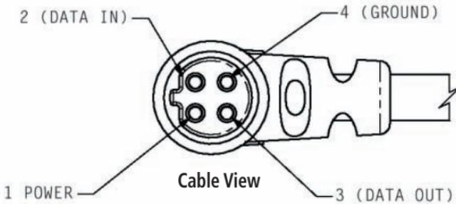
Interface formats are selected from the Setup 'Interface Page' on page 55 of this manual. See also page 68 for using the Rino with MapSource. The input/output lines on your Rino unit are RS-232 compatible, allowing easy interface to a wide range of external devices, including PC's, differential beacon receivers, marine autopilots and /or a second GPS receiver.
