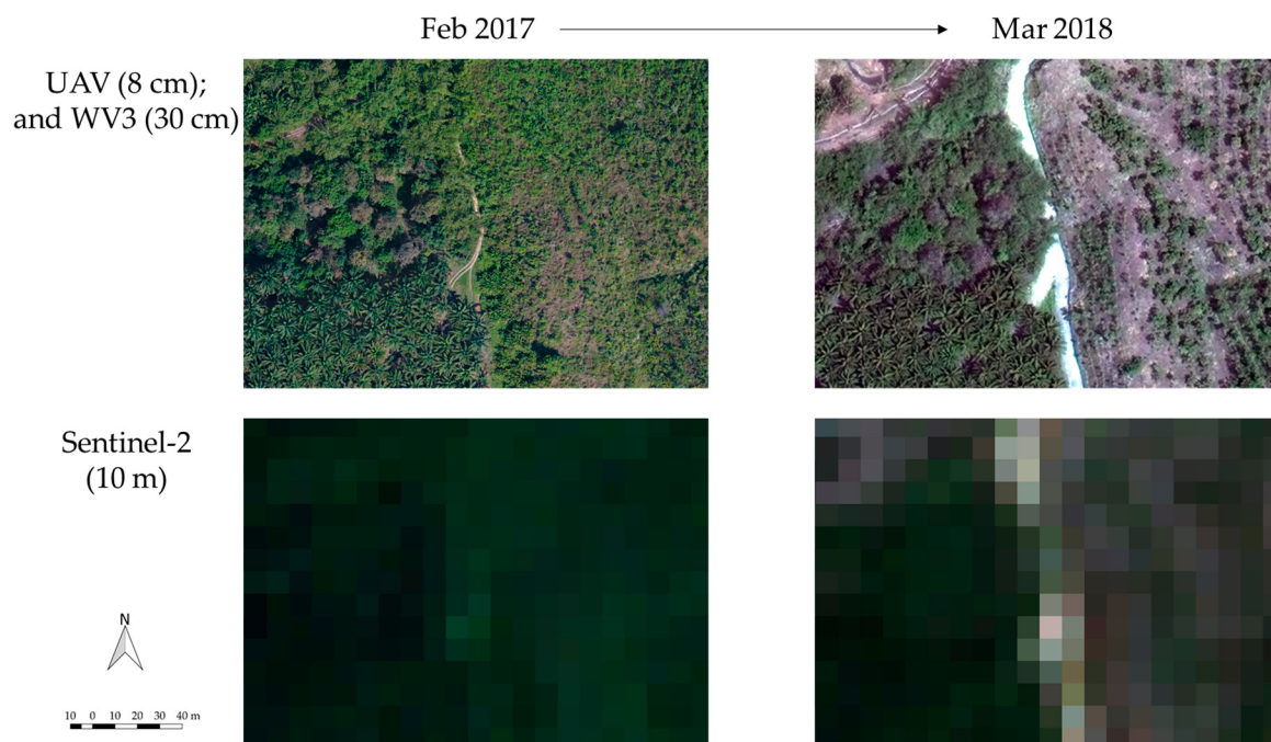
Figure 2. Examples of images of the same location using UAV, WV3, and Sentinel-2 in February 2017 and March 2018 (shown in RGB).
